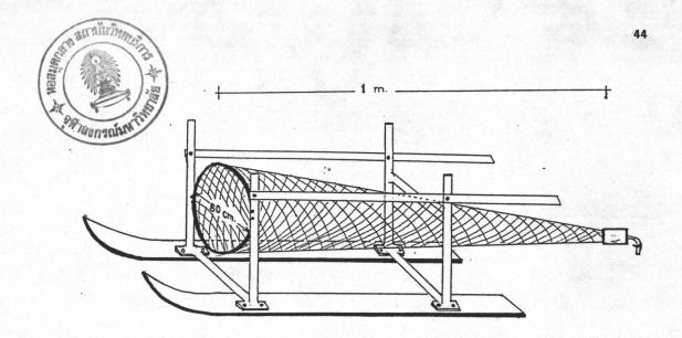
Figure 3 Modified zooplankton net for collecting zooplankton overlying the seagrass beds.
