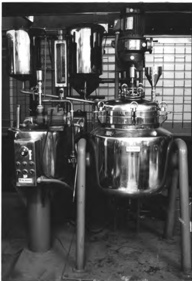
Figure 3.1 Reactor set for deproteinization of field latex
