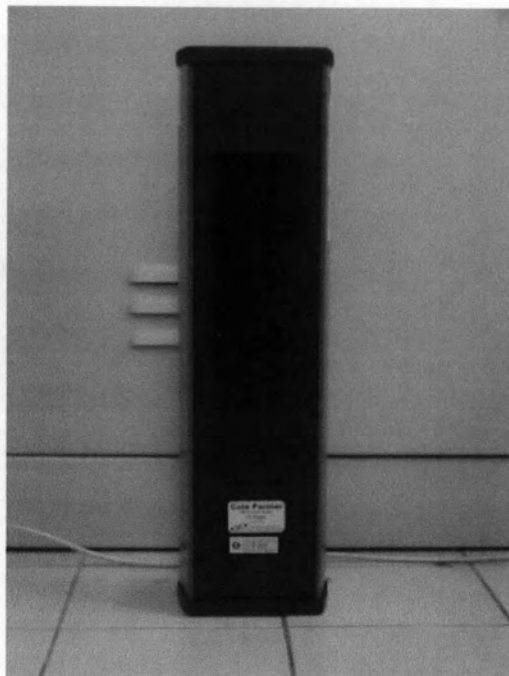
Figure 7 The UV lamp (9815 series, Cole - Palmer Instrument Company with UV lamp 2X15 watts) for polymerization study
