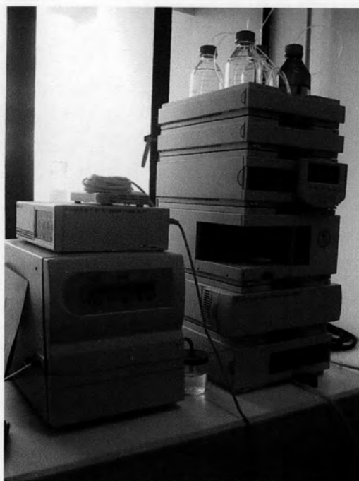
Figure 9 The High Performance Liquid Chromatography (HPLC 1100, Agilent) with UV detector without column
