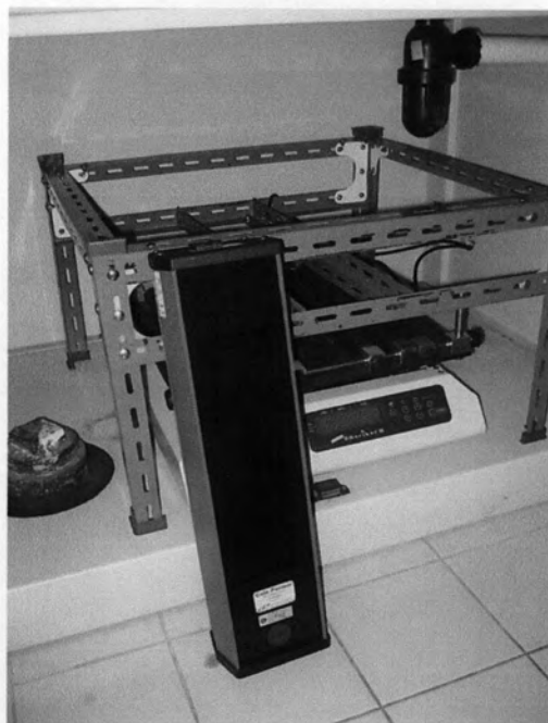
Figure 8 The polymerization system with the UV lamp (9815 series, Cole - Palmer Instrument Company with UV lamp 2X15 watts) for polymerization study
