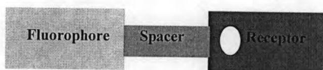
Figure 1.1 Schematic representation displaying the PET system modular design.
