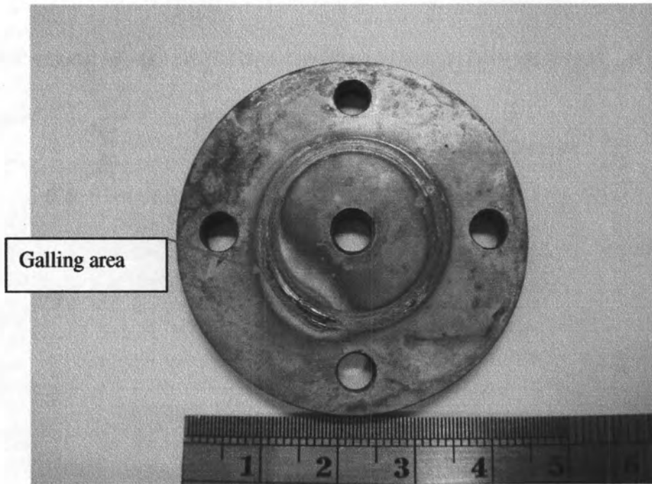
Fig. 4.19 (V,Nb)C coated disc after wear test
