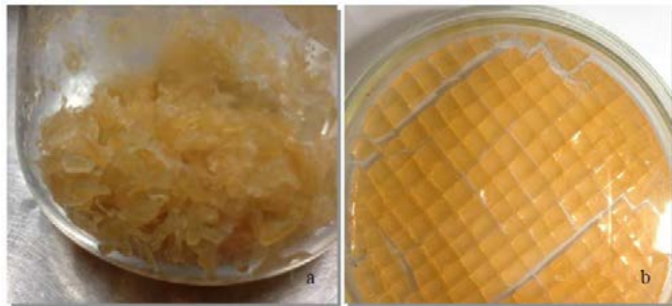
Figure 4.1 Gordonia sp. GY40 immobilized on chitosan (a) and in silica (b)
