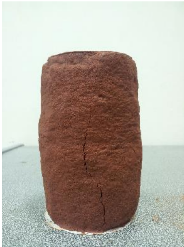
Figure 4.18: Shear failure on a CU test
