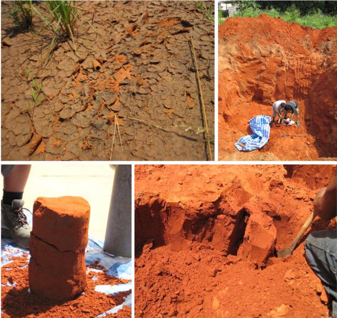
Figure 3.1: Soil Sampling. (a) The response of shredding of the soil due to evaporation in the topsoil layer and (b) shows the test pit at 2.50 meters to 3.00 meters at Khon Kaen University (c) the fragility of the soil sample (d) manual block sampling done.
