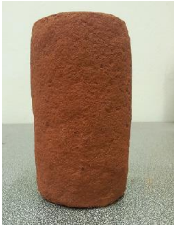
Figure 4.13: Sample after UU test
