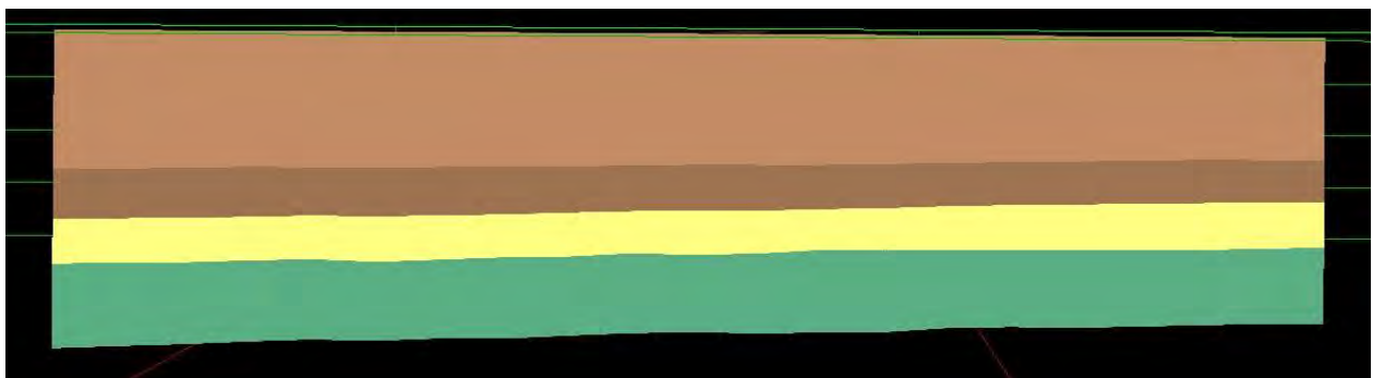
Fig 3.11 – Side section of the 3D-basin model showing 4 layers; Sequences 1, 2, 3 and overburden (Sequence 4+5).
