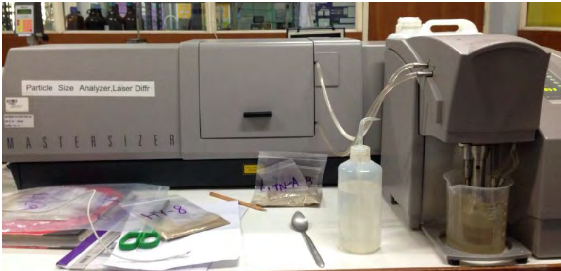
Fig.8 Particle Size Analyzer, Laser Diffraction service in Department of Industrial Chemistry, Faculty of Science, Chiang Mai University.
