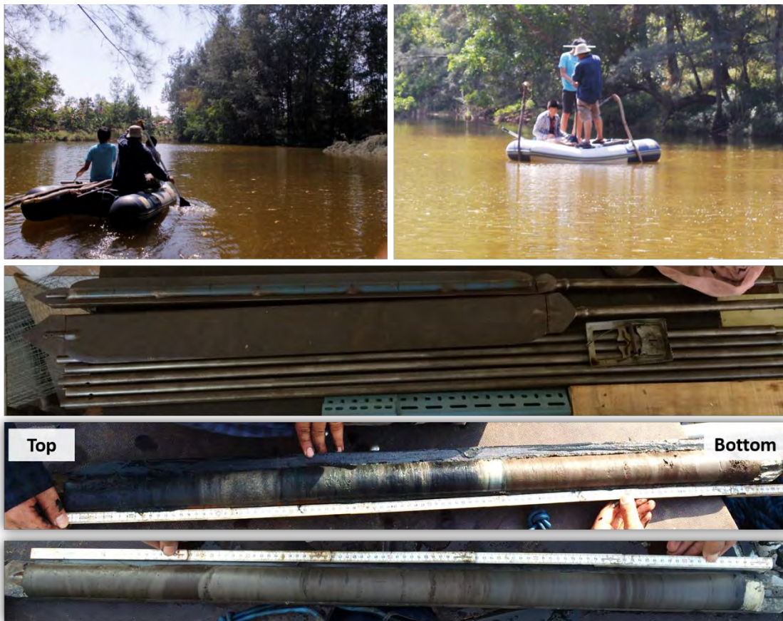
Fig.7 Coring point in lagoon (top), Russian core sampler set (middle) and sediment core samples (bottom).
