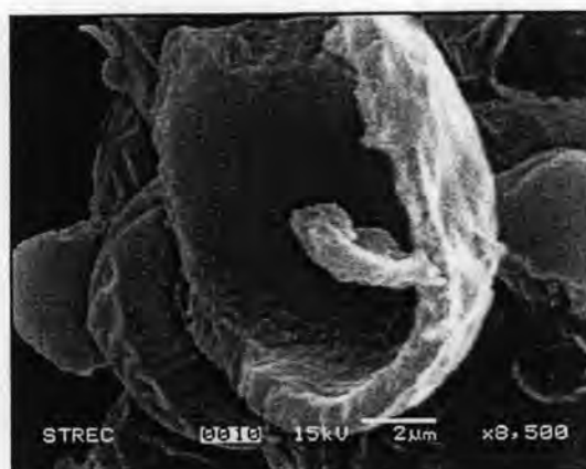
Figure 25 Scanning electron micrographs of the broken spray-dried powders with HPC/M ratio of 5:5. Magnification 8500x. Scale bar = 2 \mu\text{m} .
