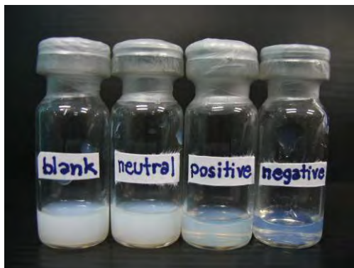
Figure 7: Physical appearances of liposomal preparations: blank = blank PC liposomes, neutral = calcein AM-loaded neutral liposomes, positive = calcein AM-loaded positively charged liposomes, and negative = calcein AM-loaded negatively charged liposomes
