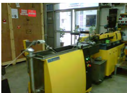
Figure 3.1 Preparation of crosslinked PLA via twin-screw extruder.
