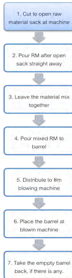
Figure 4.6.2: The new process improve for mixing process
