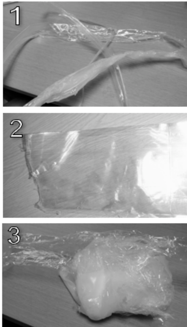
Figure 3.6.7: Three types of defect in film blowing process
