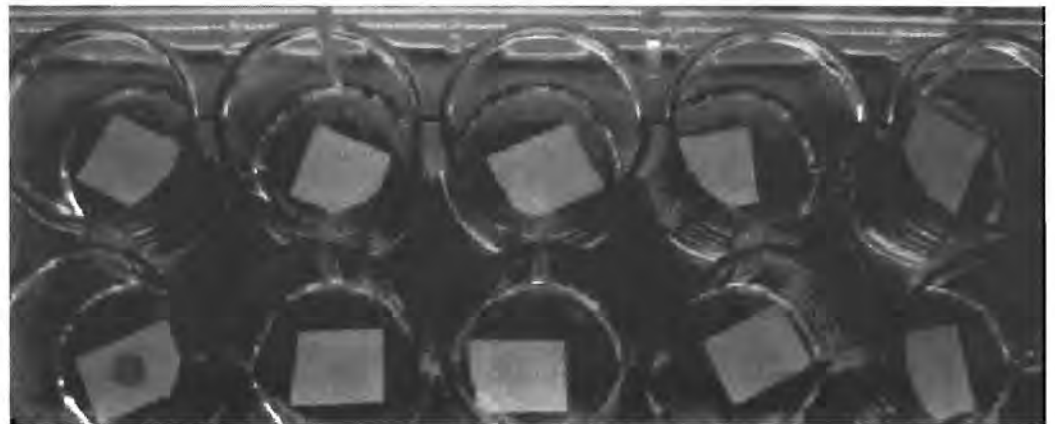
Figure 3.33 – Effect of PEG upon the final signal intensity when conjugated gold nanoparticles probes were used to detect antigen. (Upper) The sensing signal of L. pomona antibody-conjugated gold nanoparticles with PEG (Lower) Sensing signal of PEG-free conjugated gold nanoparticles.
