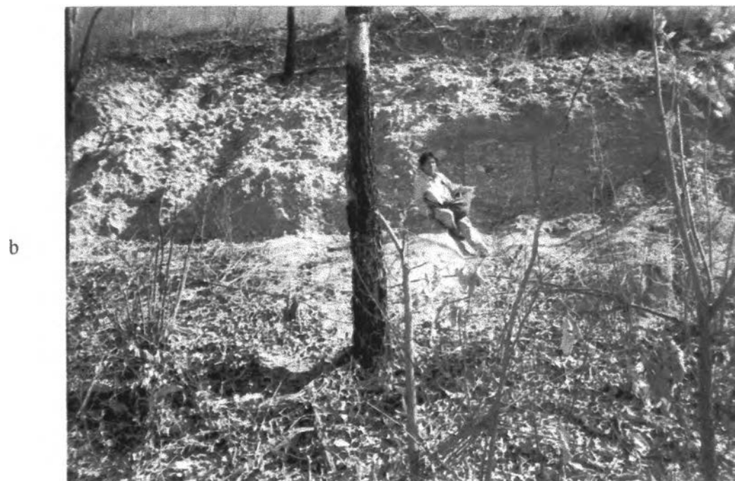
Figure 2.4 a, b Fifty stones within one square-meter of the ground or layer were selected for morphometrical gravel analysis and pebble composition analysis
