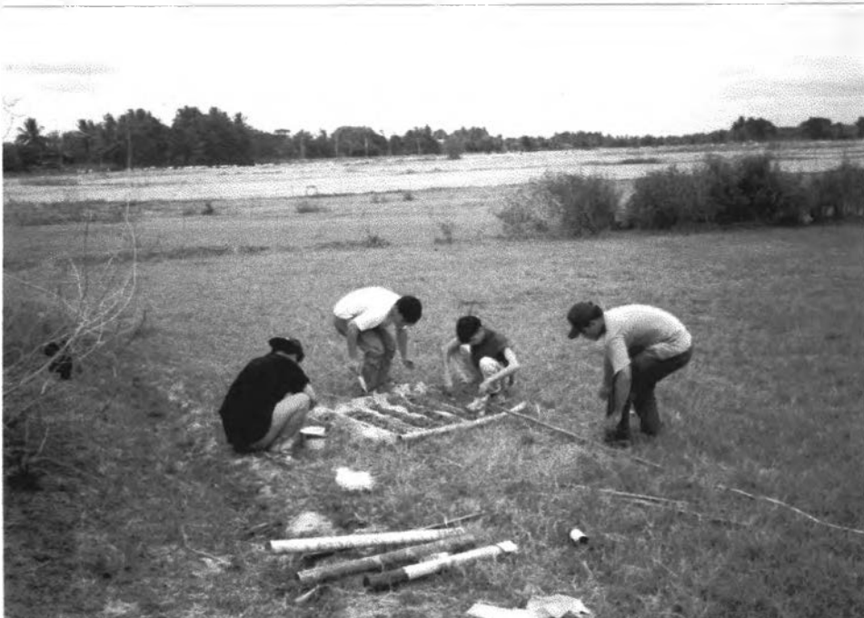
Figure 2.6 Samples from borehole were recorded and described.
