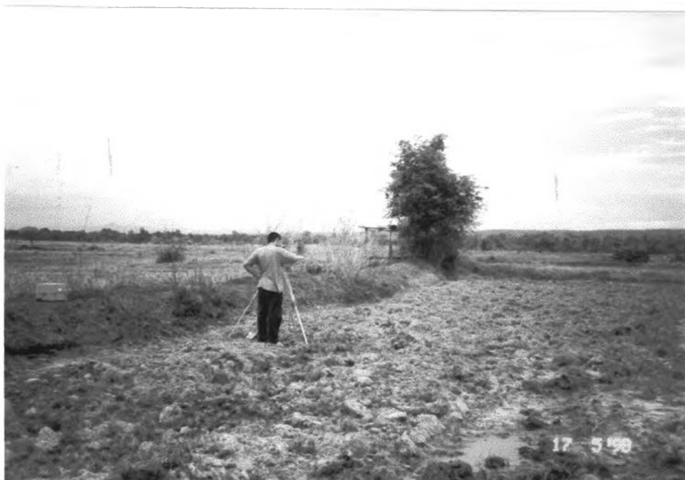
Figure 2.7 a, b Survey work to see cross section of the area, slope, width, altitude and distance from main river were measured.
