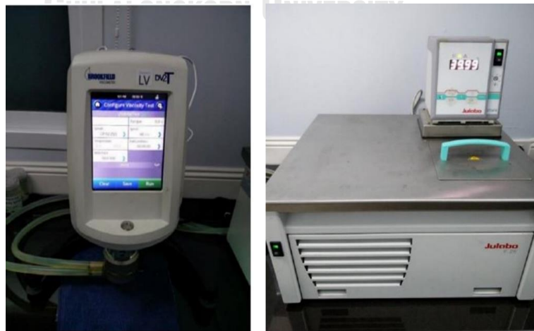
Figure 3. 1 Viscometer with temperature-controlled bath
