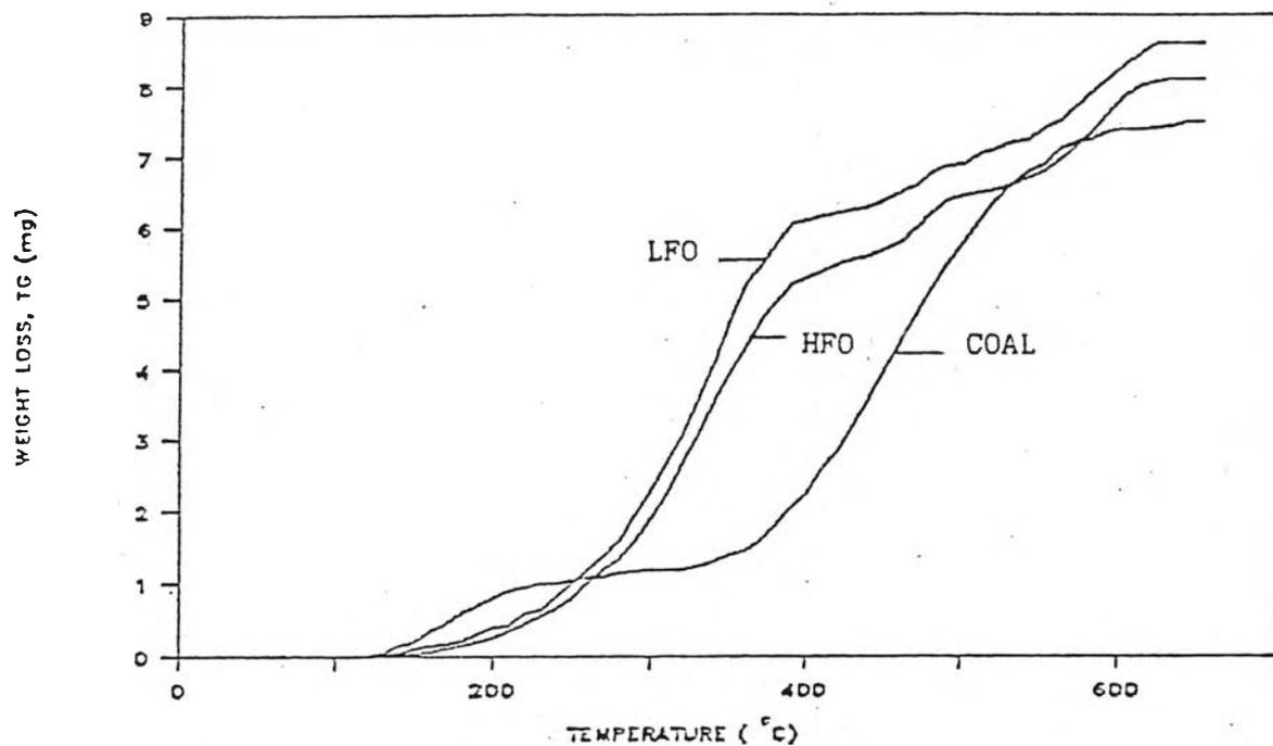
Figure 4.20 TG curve for HFO, Ban Pu coal and LFO.
