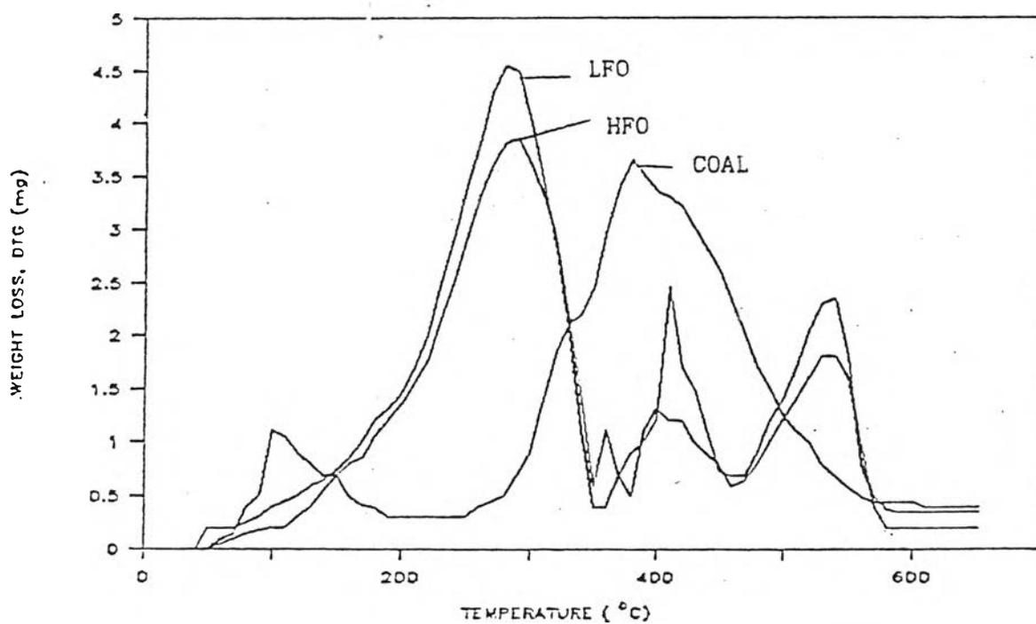
Figure 4.21 Burning profile of HFO, Ban Pu coal and LFO.
