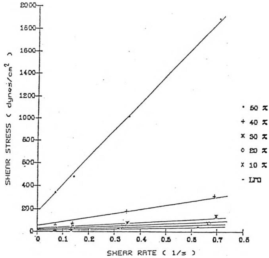
Figure 4.4 Rheogram of Ban Fu coal in light fuel oil; various coal concentrations, 40 °C.
