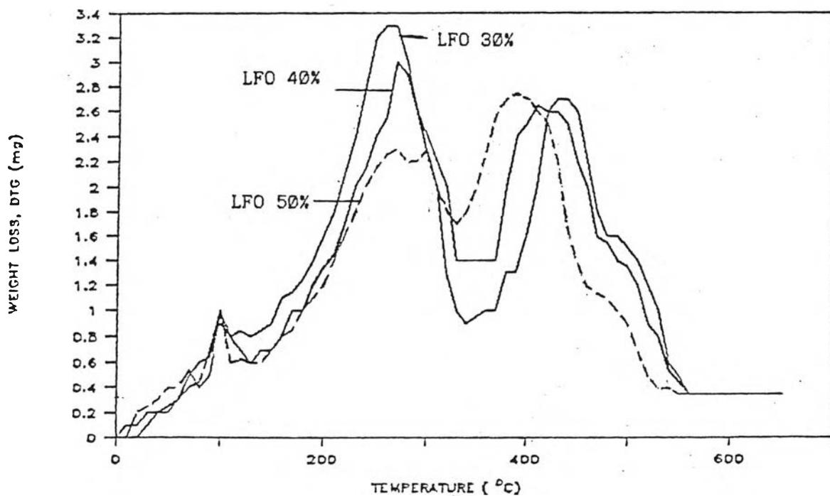
Figure 4.33 Burning profile of COM composed of 30, 40 and 50 wt% Ban Pu coal in LFO.
