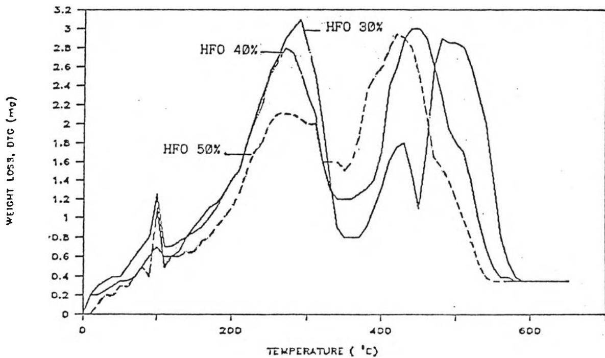
Figure 4.29 Burning profile of COM composed of 30, 40 and 50 wt% Ban Pu coal in HFO.
