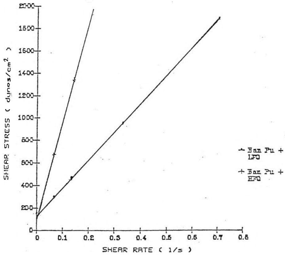
Figure 4.12 Rheogram of Ban Pu coal in different fuel oil types, 50 wt% coal and 40 °C.
