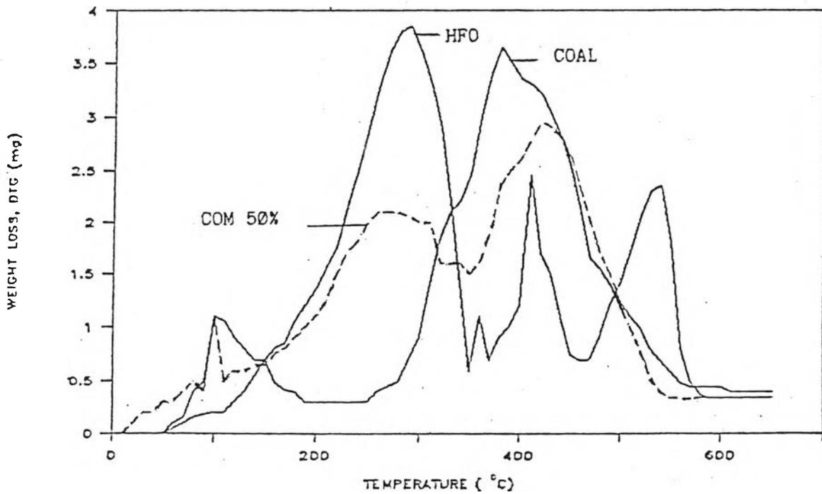
Figure 4.23 Burning profile of HFO, Ban Pu coal and COM composed of 50 wt% Ban Pu coal in HFO.
