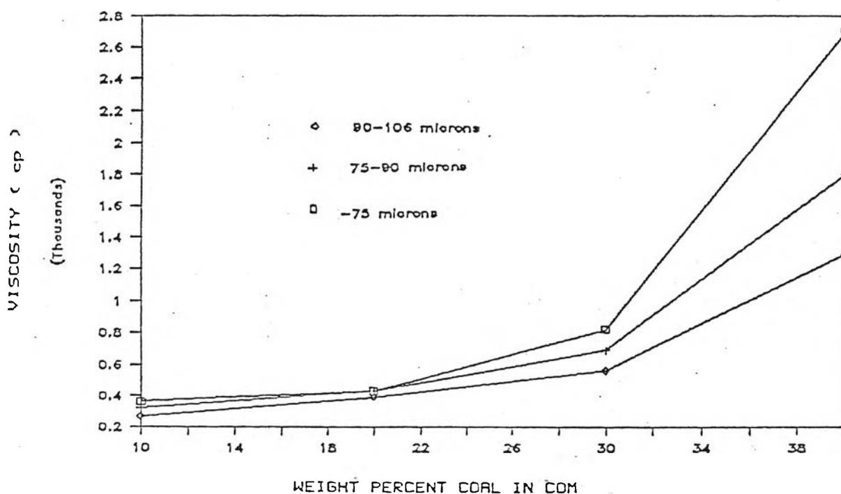
Figure 4.15 Viscosity as a function of coal concentration for Ban Pu coal and heavy fuel oil; various particles size distributions.
