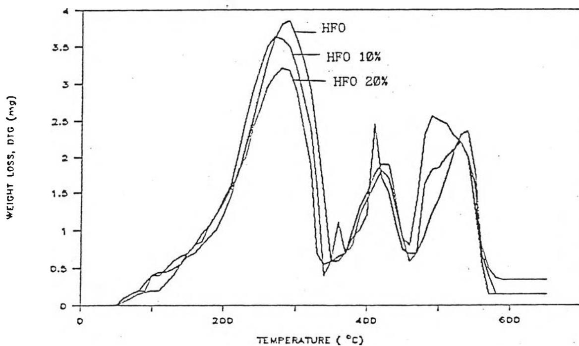
Figure 4.27 Burning profile of HFO and COM composed of 10 and 20 wt% Ban Pu coal in HFO.
