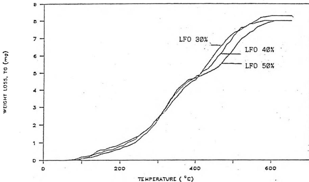
Figure 4.32 TG curve for COM composed of 30, 40 and 50 wt% Ban Pu coal in LFO.
