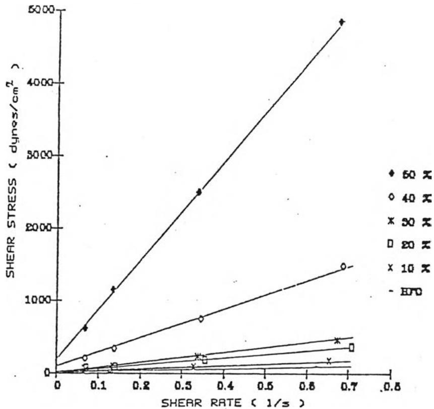
Figure 4.6 Rheogram of Mae Moh coal in heavy fuel oil; various coal concentrations, 40 °C.
