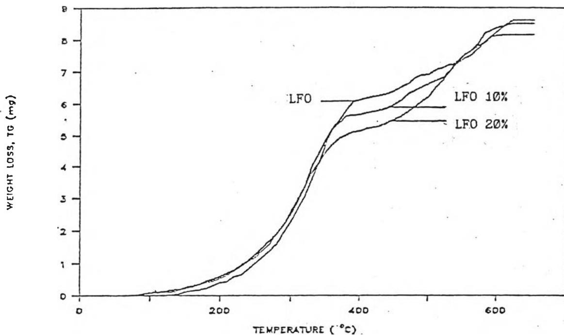
Figure 4.30 TG curve for LFO and COM composed of 10 and 20 wt% Ban Pu coal in LFO.
