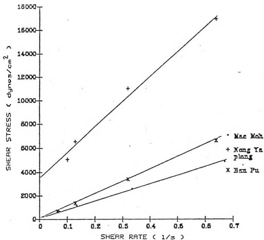
Figure 4.11 Rheogram of coal in heavy fuel oil; various coal concentrations; 50 wt% coal and 40 °C.
