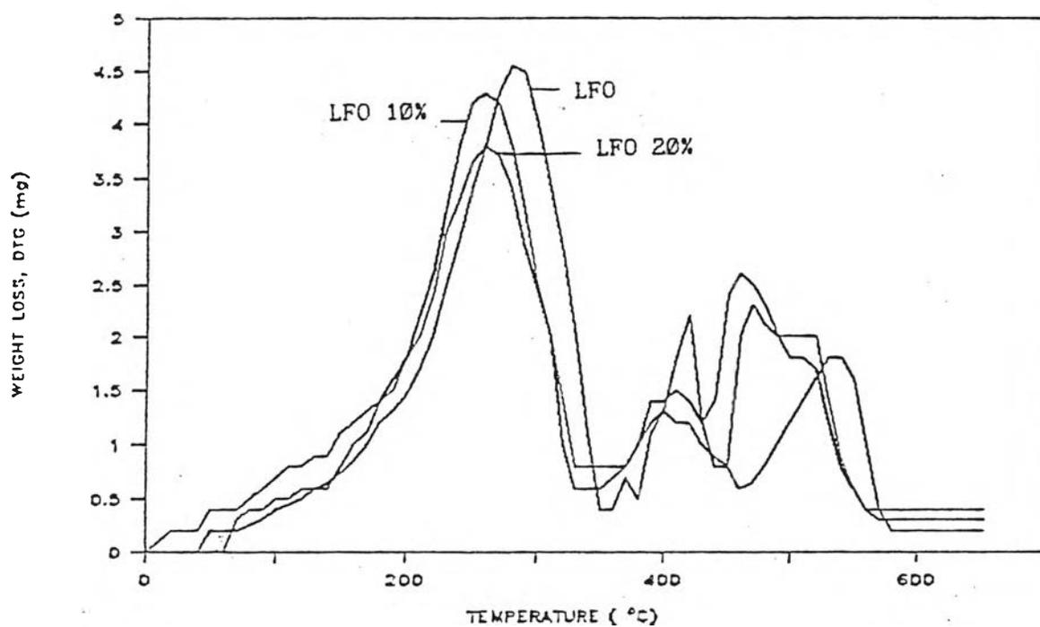
Figure 4.31 Burning profile of LFO and COM composed of 10 and 20 wt% Ban Pu coal in LFO.
