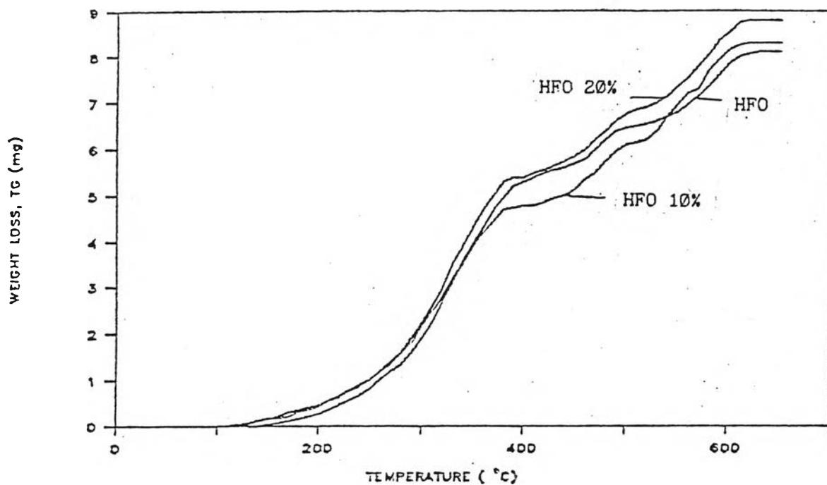
Figure 4.26 TG curve for HFO and COM composed of 10 and 20 wt% Ban Pu coal in HFO.
