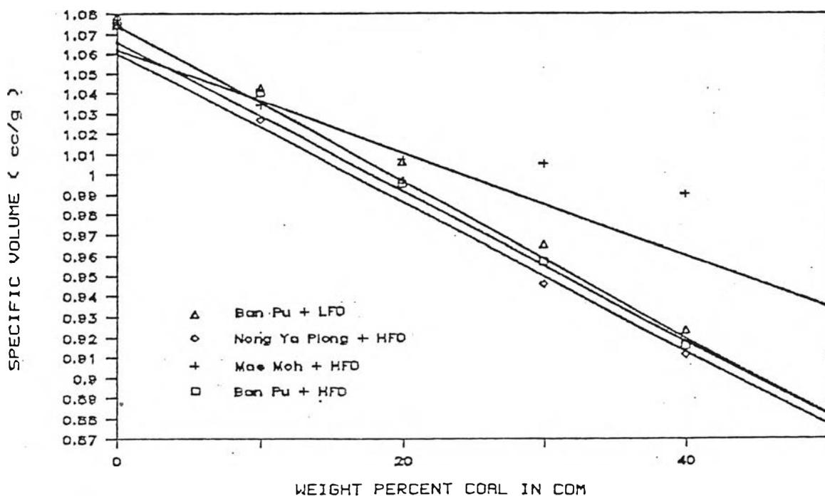
Figure 4.16 Specific volume of typical Coal-Oil Mixture.
