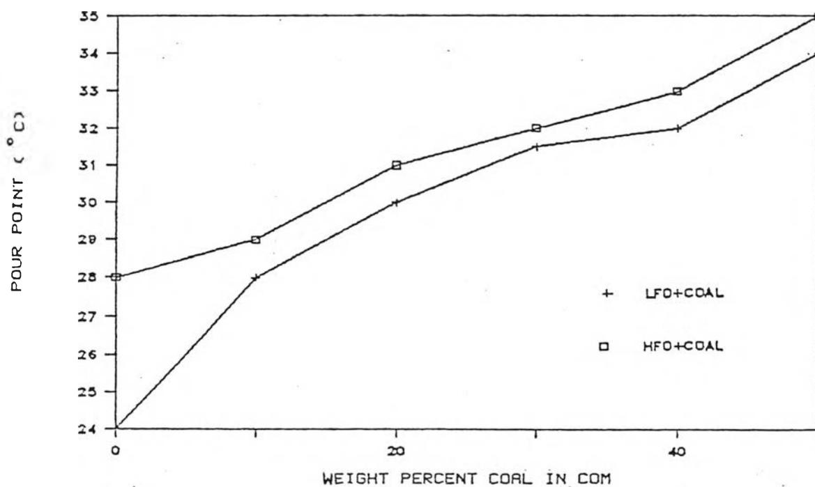
Figure 4.1 Variation of pour point with coal concentration for Ban Pu coal in different fuel oil types.
