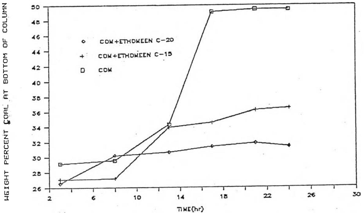
Figure 4.17 Weight percent coal at bottom of column as a function of time for 25 % COM Ban Pu coal in light fuel oil measured with the sedimentation column for different additives.
