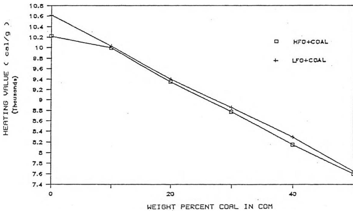
Figure 4.3 Variation of heating value with coal concentration for Ban Pu coal in different fuel oil types.
