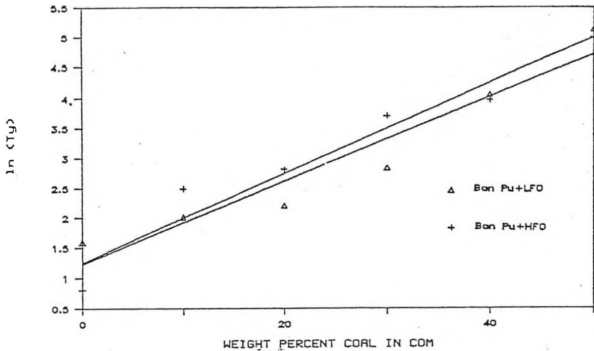
Figure 4.8 Dependence of yield stress on coal concentration; different fuel oil types, Ban Pu coal and 40 °C.
