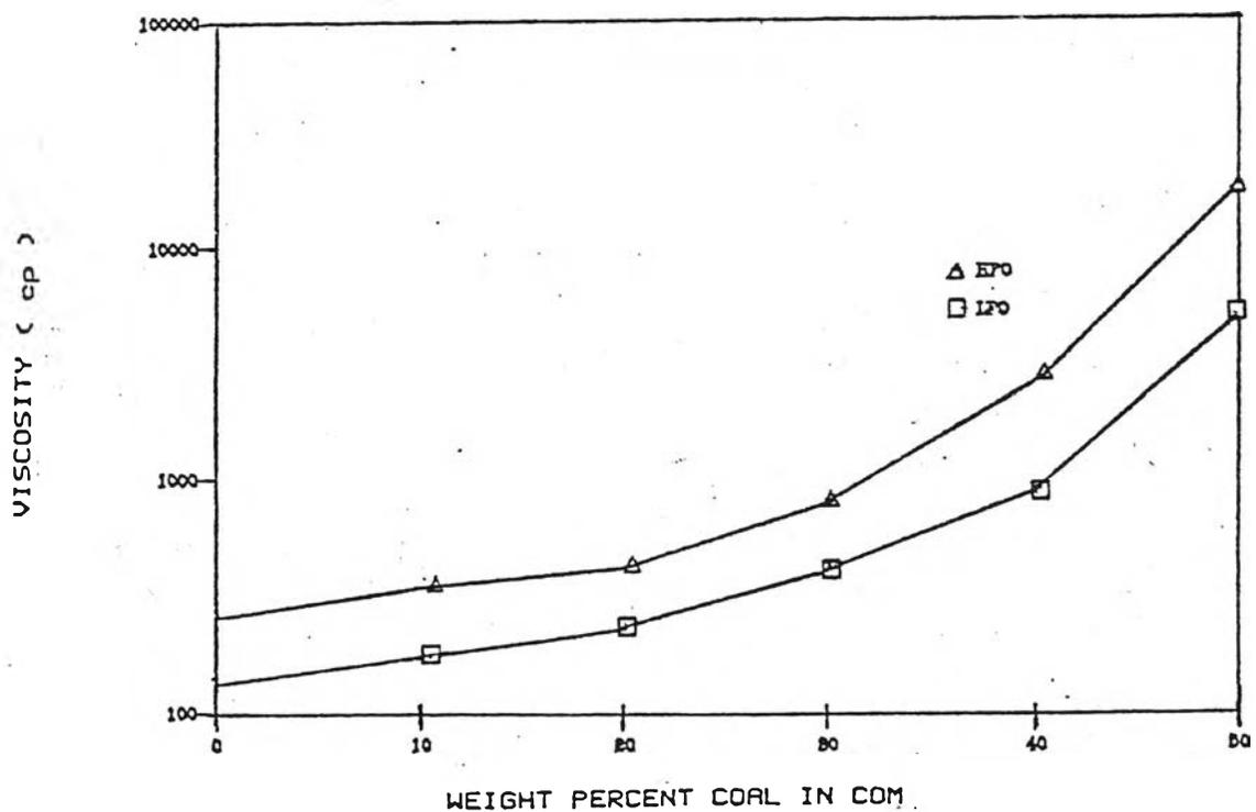
Figure 4.14 Viscosity as a function of coal concentration for Ban Pu coal and different fuel oil types.
