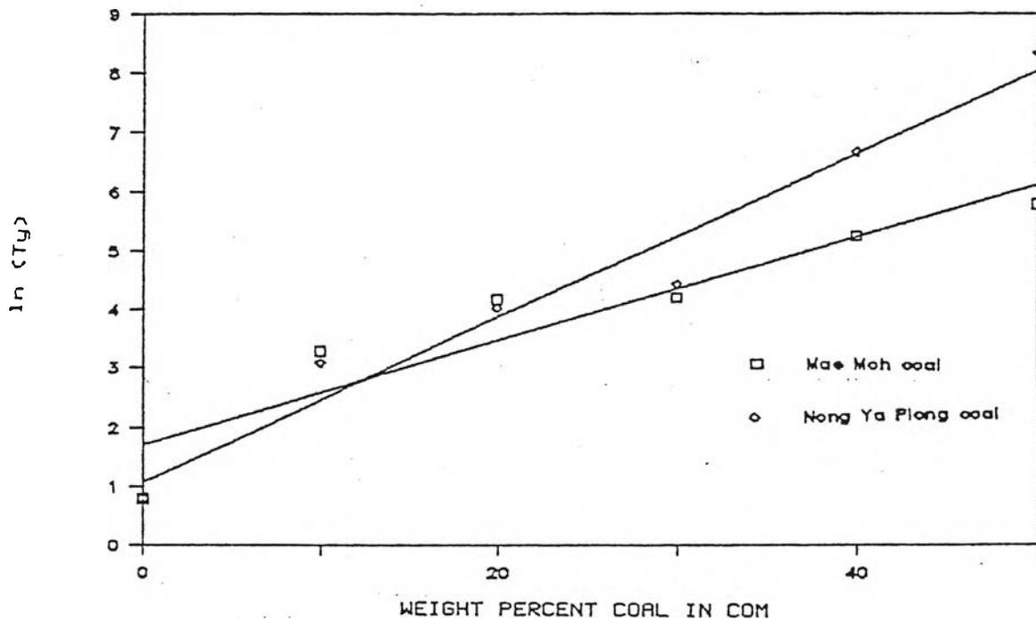
Figure 4.9 Dependence of yield stress on coal concentration; various coal types, heavy fuel oil and 40 °C.
