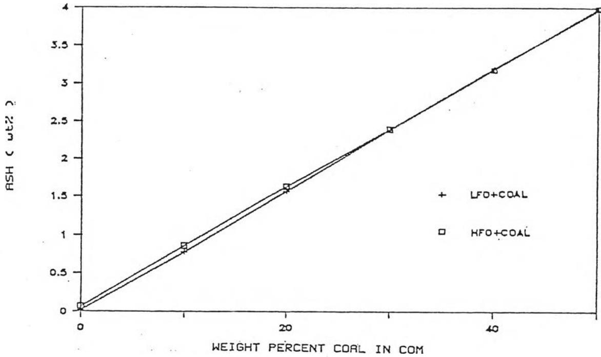
Figure 4.2 Variation of weight percent ash with coal concentration for Ban Pu coal in different fuel oil types.
