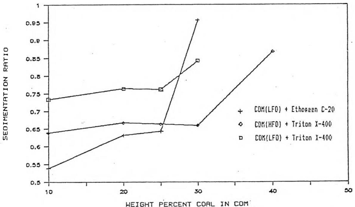
Figure 4.18 Sedimentation ratio as a function of weight percent coal for Ban Pu coal in light fuel oil and heavy fuel oil with two additive types.
