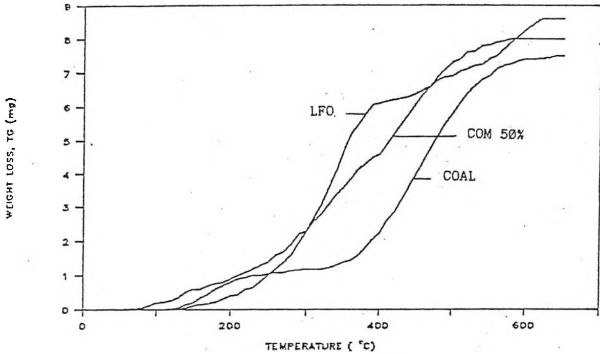
Figure 4.24 TG curve for LFO, Ban Pu coal and COM composed of 50 wt% Ban Pu coal in LFO.
