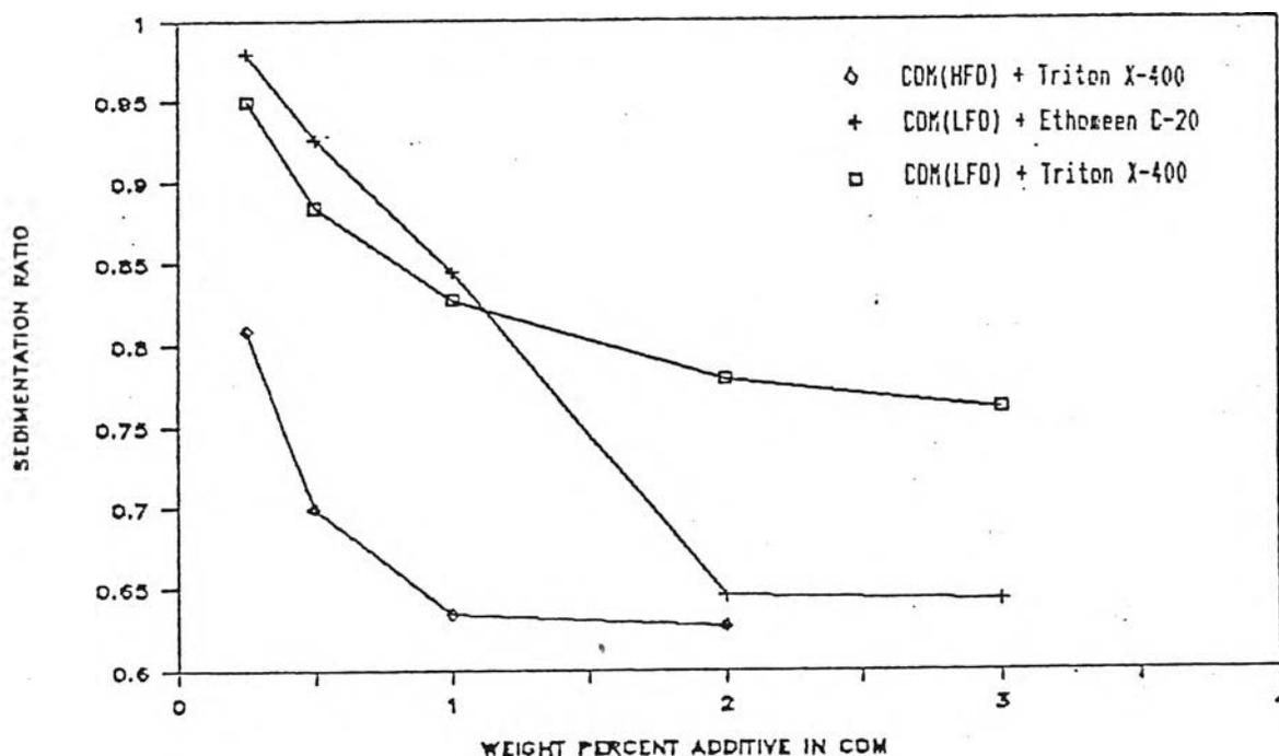
Figure 4.19 Sedimentation ratio as a function of weight percent additive for Ban Pu coal in light fuel oil and heavy fuel oil with two additive types.
