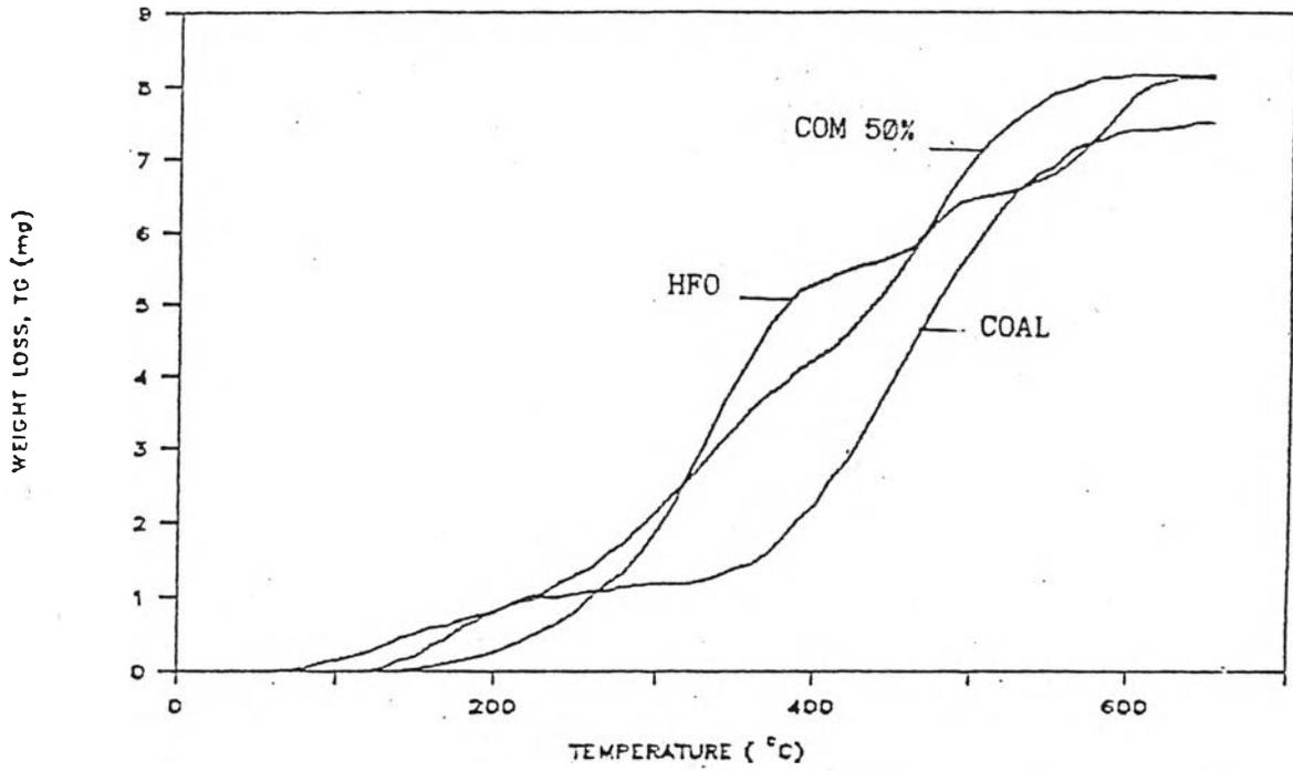
Figure 4.22 TG curve for HFO, Ban Pu coal and COM composed of 50 wt% Ban Pu coal in HFO.
