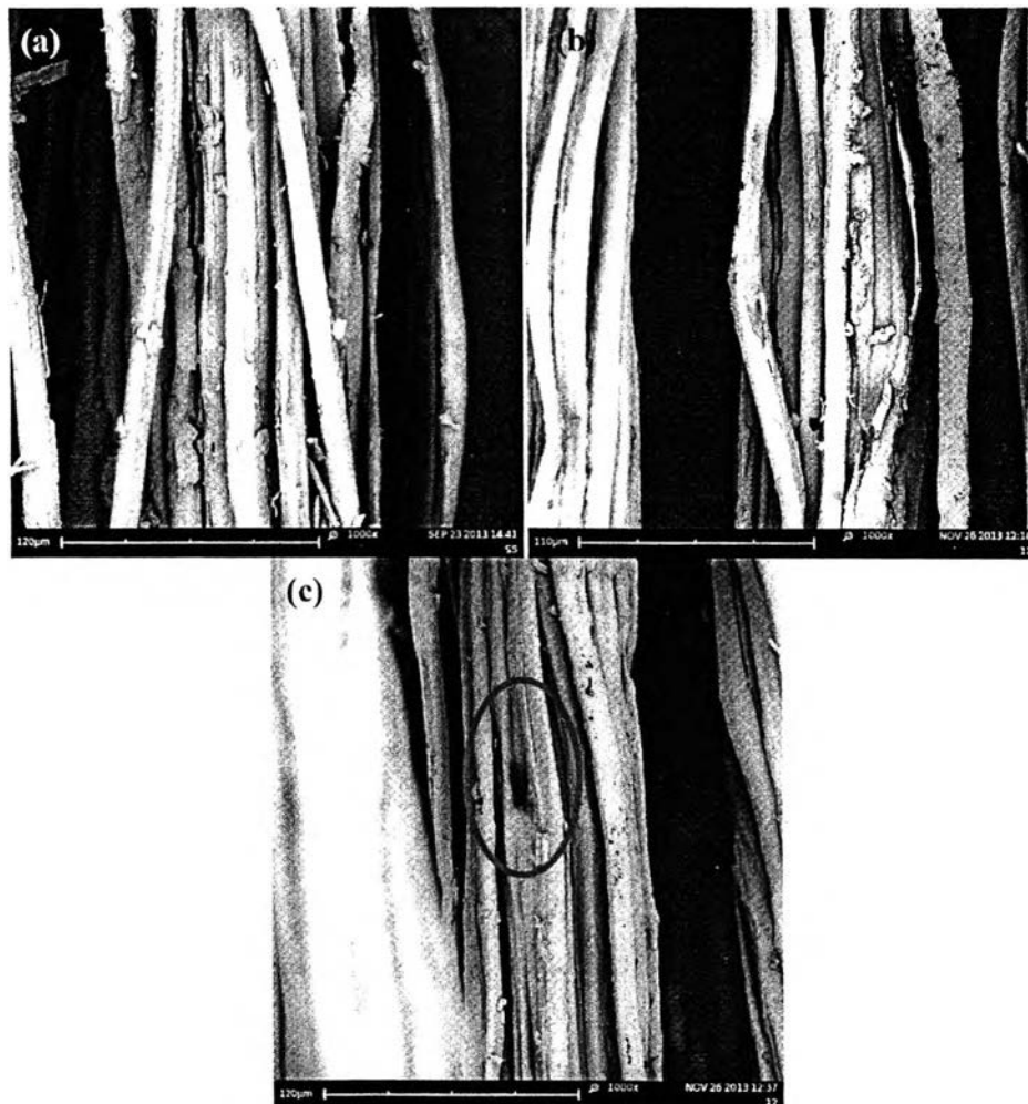
Figure 4.13 SEM micrographs of silk fibers treated by plasma. Condition: discharge power at 2000 Watt, exposure time at 10 min and oxygen flow rate at 500 cc/min. and varying chamber temperature (a) 25 °C. (b) 50 °C and (c) 75 °C
