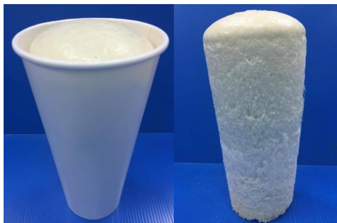
Figure 3.1 RPUR foams prepared by the cup test method and catalyzed by \text{Zn(OAc)(Val)} (1:1)
