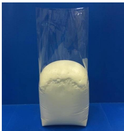
Figure 3.2 RPUR foams prepared by plastic mold method and catalyzed by Zn(OAc)(Val) (1:1)
