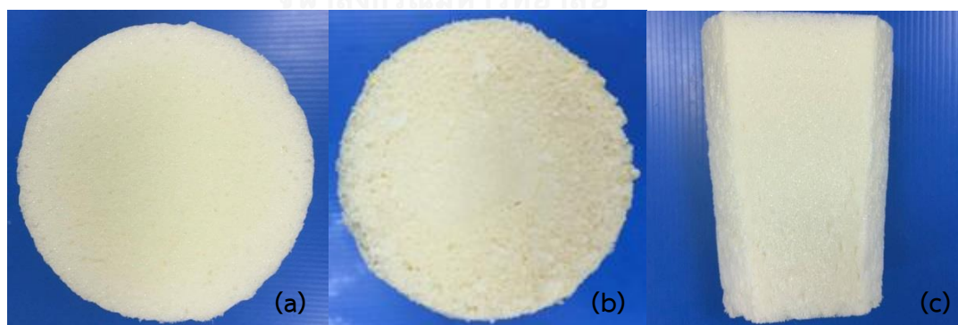
Figure 4.50 RPUR foams catalyzed by Zn(OAc)(Val) (1:1) (a) top; (b) bottom; (c) side of the foam sample
