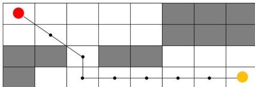
Figure 5.40. The concept of obstacle avoidance system using A* algorithm.
