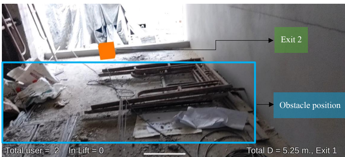
Figure 7.34 Example of the output in case it is impossible to walk through due to obstructions.
